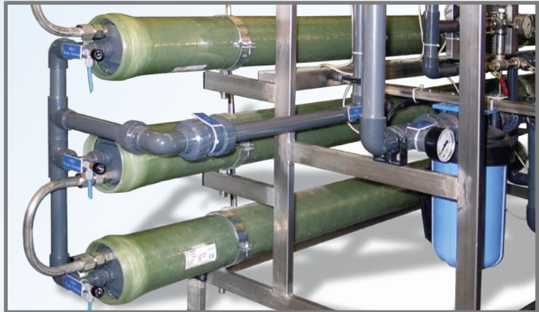
W.E.T. - Reverse Osmosis System
